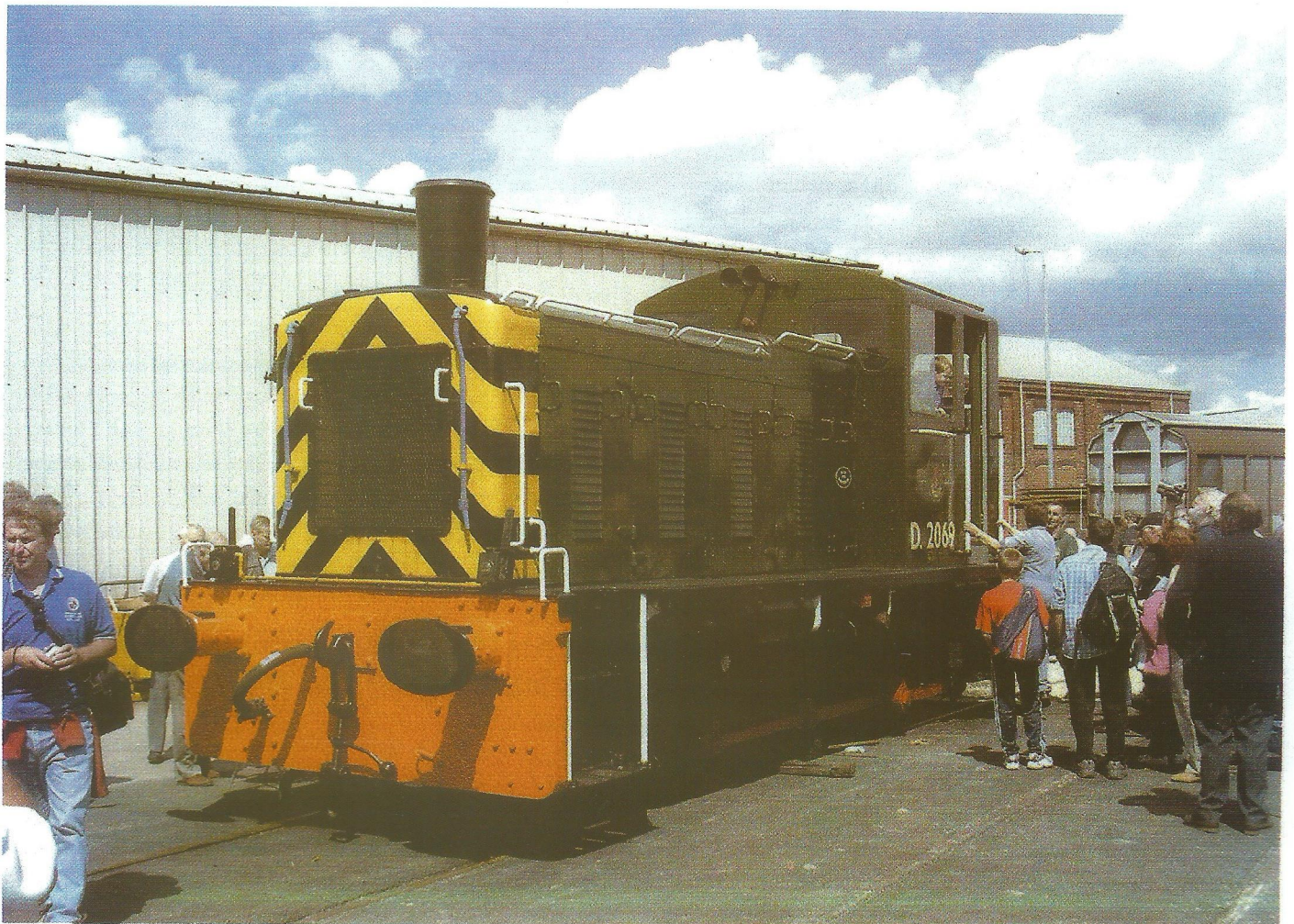
A diesel mechanical shunter ( below ), class 03, Number D2069, one of the Plant's smaller locomotive products built in 1959, withdrawn from service in 1983.
